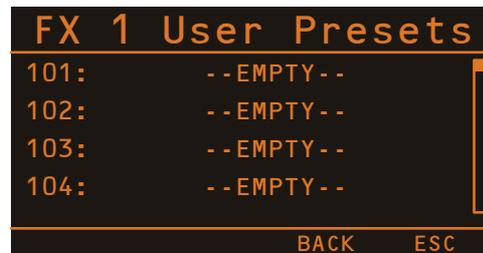
Turn the MENU/ENTER rotary encoder to select the user preset where the edited effect should be stored. Press the MENU/ENTER rotary encoder to open the Set FX Name dialog.
