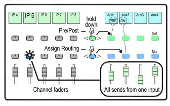
Press an Input Channel strip Mix key.
