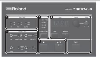
Switches the synchronization signal setting (SYNC 24, SYNC 48) of the DIN SYNC connectors (IN, OUT 1, OUT 2).
