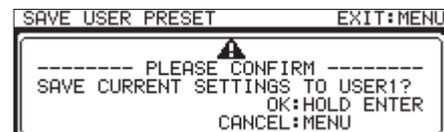
3. When the confirmation message is open, press and hold the **MULTI JOG** dial to begin saving the user settings to the built-in memory.
