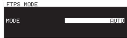
Set the mode used for SSL encryption of data sent and received by FTP on the **FTPS MODE** screen.
