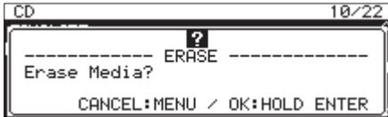
3. Press and hold the **MULTI JOG** dial to start erasing the disc.
