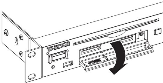
2. Inserted SD cards with the correct orientation. The label should be up and the connector should be inserted toward the back.
