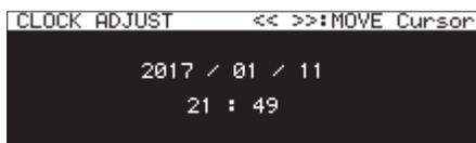
2. Press the **MULTI JOG** dial to enter setting mode and show the cursor on the item to be changed. Use the **<< [A-B]** and **>> [INPUT]** buttons to move the cursor.
