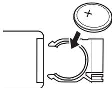
3. Insert the battery holder into the remote control.
