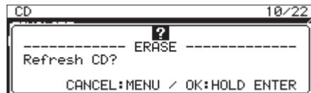
4. Press and hold the **MULTI JOG** dial to start refreshing (completely erasing) the CD-RW disc.
