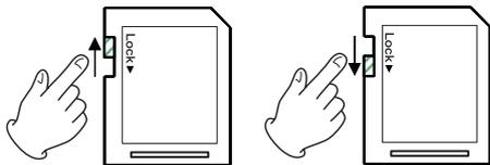
If you slide the protect switch to the LOCK position, file recording and editing will not be possible. Unlock cards to enable changing their data, including recording and erasing.
