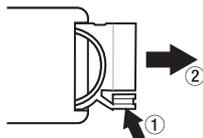
2. Being careful to maintain the correct  $\oplus$  /  $\ominus$  orientation, install the lithium coin battery (CR2025) into the battery holder.
