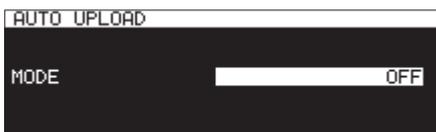
Set the **AUTO UPLOAD** screen to automatically upload files that have completed recording to the FTP server.
