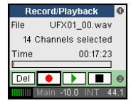
Playback mode turning encoder 2 allows to change the current playback position.
