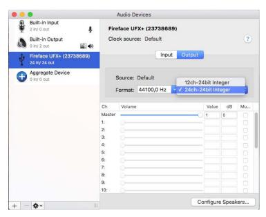
Mac OS X supports USB Audio 2.0, even with more than 2 channels. The UFX+ offers 24 input and 24 output channels at up to 96 kHz. It is shown as "Fireface UFX+ (xxxxxxxx)" in the Audio MIDI Setup, in both normal and CC mode. In CC mode the USB Settings will vanish from the Dock, and TotalMix will – if at all – show a 'disconnected' UFX+.
