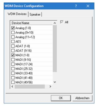
The screenshot to the left shows the multichannel WDM devices available with the UFX+ after selecting 'Multi-Channel' in the WDM Devices listbox and hitting WDM Configure. In this example the devices Analog 1 to 8 and MADI 1 to 8 are active.
