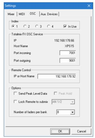
➤ **Number of faders per bank.** Available choices are 8 (default), 12, 16, 24, 32 and 48. Note that when working in underperforming networks, especially wireless, a higher number of faders might not work as smooth as expected.
