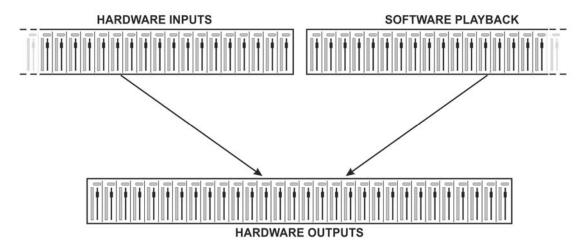
TotalMix can be used in the above view (View Options **2 Rows**). However, the default is a vertical alignment in three rows as known from an Inline desk, so that the row *Software Playback* equals the *Tape Return* of a real mixing desk:
