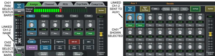
Figure 4.7b: Ch1-2 are linked, sent to Aux1, assigned to Main mix
