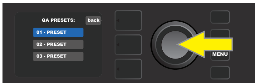
Use the ENCODER to scroll to and select one of the three QUICK ACCESS preset slots.
