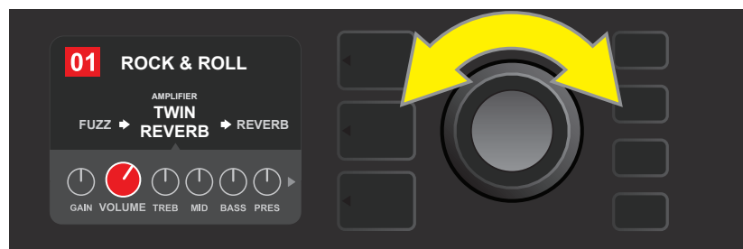
Turn the ENCODER again to adjust the selected amp model control knob to preference.
