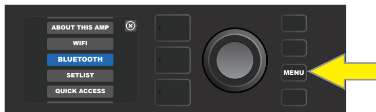
To enable Bluetooth, first press the MENU utility button.
