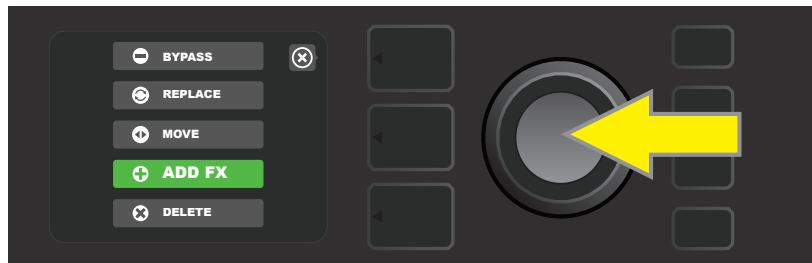
Select "ADD FX" in the effects placement options menu by scrolling to it and pressing the ENCODER.
