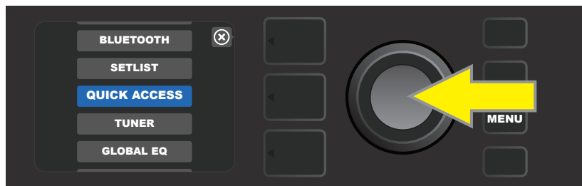
Use the ENCODER to scroll to and select “QUICK ACCESS.”
