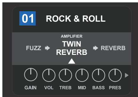
Flanked by two effects, the amp model within the preset is selected here in the SIGNAL PATH LAYER, as indicated by the white arrow and the word “amplifier.”
