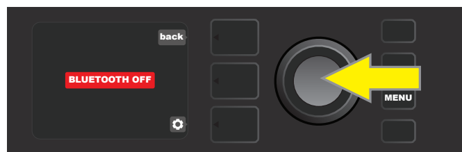
The default Bluetooth setting is "off" (labeled in a red box); press the ENCODER to turn Bluetooth on (labeled in a green box).
