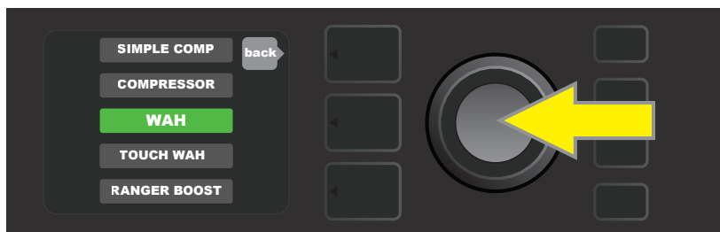
Select an effect by scrolling to it and pressing the ENCODER.
