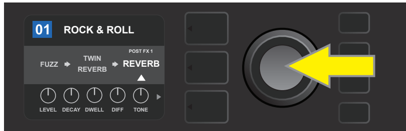
In another way to add an effect, highlight an existing effect within a preset by turning the ENCODER to it and pressing the ENCODER to see a menu of four effects categories.
