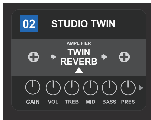
Close-up detail—of a different preset that doesn't include one or more effects—in which open slots that effects can be placed in are marked by a placeholder symbol consisting of a plus sign in a circle at both ends of the SIGNAL PATH LAYER.
