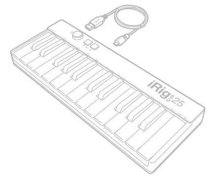
iRig KEYS 25 is a compact and portable MIDI keyboard that sports 25 velocity-sensitive mini keys – 2 full octaves for Mac/PC. It's been designed to be extremely portable and with all the necessary features, like: Volume/Data knob freely assignable and Octave/edit buttons. iRig KEYS 25 is MIDI and USB class-compliant, meaning it works with hundreds of music creation apps on Mac and PC, with no drivers to install. iRig KEYS 25 is USB powered.
