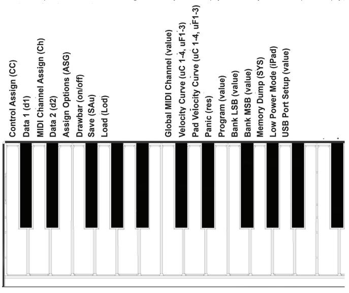
Menu keys are the same for both Impact LX49+ and LX61+ but value entry using the keyboard is one octave higher on LX61+. Refer to the screen printing on the unit to see which keys to press, to enter values.
