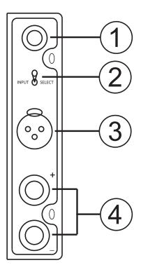
Note: Each Amplifier Module channel has separate Balanced and Unbalanced inputs and an independent Input Selector switch.
