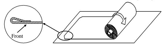
**Step 9:** Carefully and gently place the assembled frame on top of the screen material. Make sure to not allow the angle edge of the frame to come in direct contact with the screen material to avoid puncturing it.
