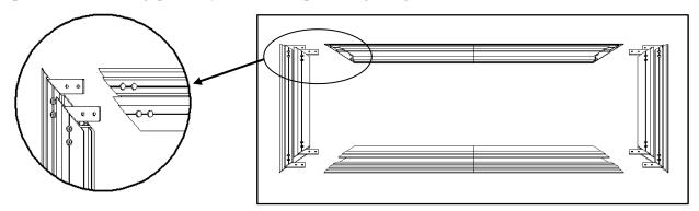
Step 7: Secure the elbow joints by fastening them with M4x6 screws (c), 4 at each corner.
