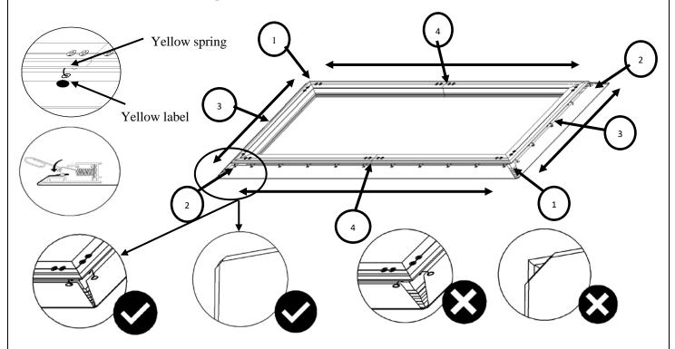
To avoid ripples forming in the material it is imperative that all of the corners are properly wrapped around the edges as illustrated in the check mark diagrams.
