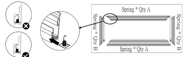
Note: The springs are pre-installed into the grooves of the frame.
