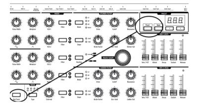
Panel + Kbd Track - Auto-tunes the instrument. Because voltages drift over time
