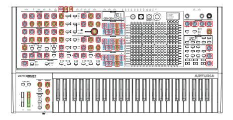
In the graphic above, the numbers superimposed over knobs are all MIDI Continuous Controllers (CC), so for example the Modulation wheel sends/receives MIDI CC#1, and Macro knob 1 to its right sends/receives CC#11 (Expression).
