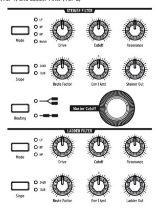
Filters remove frequencies from the sound sources coming from the Mixer see Mixer Section [p.28], and they are a primary component in the subtractive synthesis technique used by the MatrixBrute and all analog synths. Modulating them varies the timbre of the sound over time. With very high Resonance levels they can self-oscillate, becoming another sound source.
