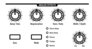
The operation instructions cover the MatrixBrute's Analog Effects [p.34] in detail, but just to "finish" the sound and bring this module to your attention, turn the Wet/Dry knob up a little to add some space. Use the Mode button to try other effects.
