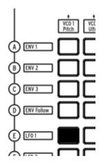
LFO 1 is five rows down, VCO 1 Pitch is the first column, so simply push the button where the two intersect. The button lights purple, indicating it's the one that's selected; if you click on another button to select additional modulation routings, it'll turn blue to show it's been assigned.
