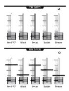
Envelopes shape voltage levels over time while you're triggering a note on the keyboard. While it can be routed to additional places in the MOD Matrix (see below), ENV 2 is always hardwired to control the MatrixBrute's VCAs. VCA stands for voltage-controlled amplifiers, which means all the sound sources that appear in the Mixer, i.e. the VCOs and/or any external signals plugged into the back of the instrument.
