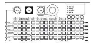
The **MOD**ulation Matrix is an electronic patchbay that routes all the MatrixBrute's modulation sources to any or all possible destinations. Think of this as a grid of patch cords, each with an attenuator that allows for positive or negative modulation. Every parameter that it would make sense to modulate - pretty much anything with a knob or fader - can be a destination.
