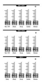
Envelopes are adjustable modulators that shape the voltage over time. MatrixBrute has two 4-stage, ADSR (Attack Decay Sustain Release) envelopes, plus a third one (ENV 3) which adds a Delay phase before the ADSR (this is all explained below). Each envelope has a "gate" LED that show when a gate is receive and will fade out to show when the release stage is still active.
