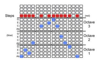
You can hold down any four notes (or fewer), in the example above, Ab-C-E-G are being arpeggiated in the pattern shown, use the blue buttons to shift the specific note of your arpeggio up or down within the three octaves. The red line shows the steps, i.e. the rhythm pattern.
