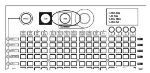
Press the MOD button. The Matrix becomes an electronic patchbay.
