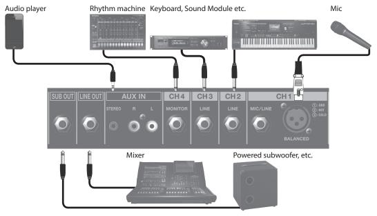
\* To prevent malfunction and equipment failure, always turn down the volume, and turn off all the units before making any connections.
