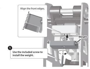
\* After installing the weight, make sure that the screw is tight.
