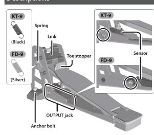
\* Do not touch the sensor area or insert a foreign object into it. Doing so will cause faulty operation or malfunction
