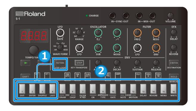
1. Hold down the [PATTERN] button and press the [1]-[4] pads to select a bank.
