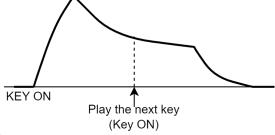
If "PaL 9" is selected while the unit is in POLY mode, time-based changes are applied to the volume or tonal quality of each note you play, regardless of whether you play in a legato or non-legato style.
