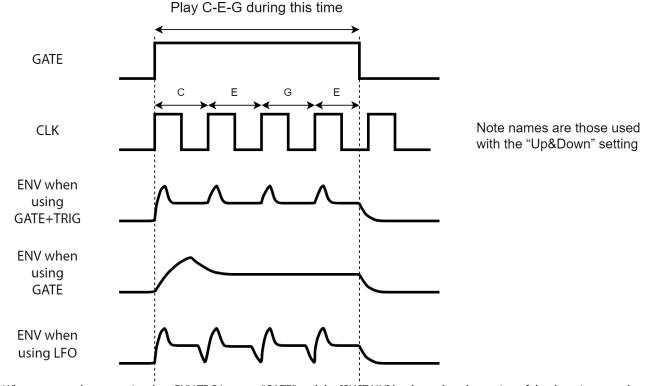
When you use the arpeggio when ENV TRG is set to "GATE" and the [SUSTAIN] knob reaches the setting of the decaying sound (0), the sound stops as the envelope ends.
