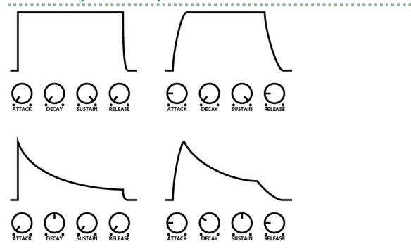
When the [ATTACK] knob, [DECAY] knob, [SUSTAIN] knob and [RELEASE] knob are all set to "0", an extremely short pulse wave is generated, producing a click noise.
