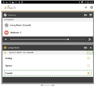
5. The just selected Input (Coaxial) can now be streamed to the Wireless Loudspeakers (Bedroom 1) and can also be listened to in the Living Room (via the MB50). Referring to figure 44 make the appropriate room selections followed by selecting "DONE".
