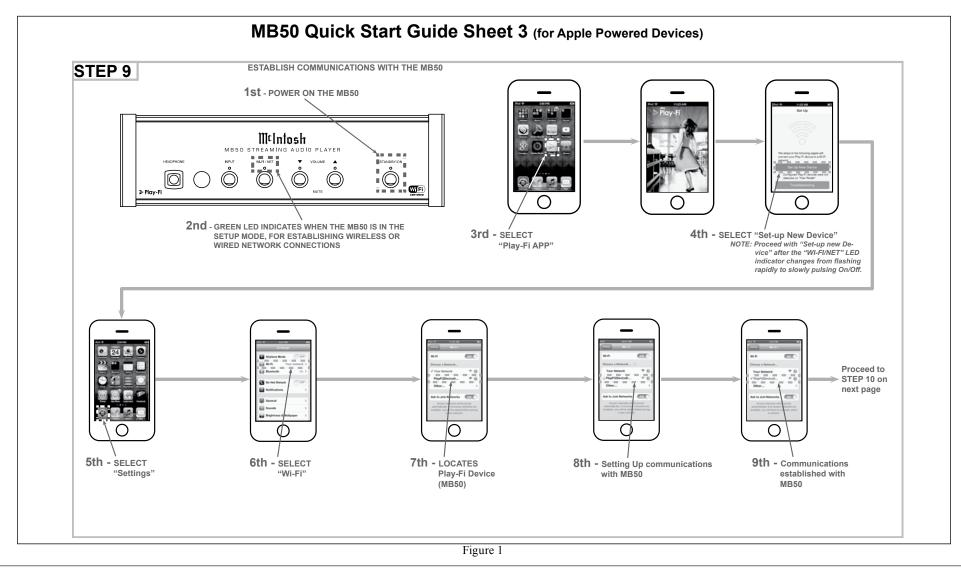
The MB50 Quick Start Guide (located on the supplied separate folded sheets) will aid in establishing the communications between the MB50, your Mobile Device and the Network/Wireless Router. Figures 1 and 2 are sample illustrations from the MB50 Quick Start Guide for Apple and Android Powered Mobile Devices. After communications have been established, proceed to page 16 "How to Operate the MB50".
