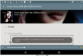
4. The music selection that has the unsupported sample rate may be listened to by switching Off the Critical Listening Mode. Switch Off the Critical Listening Mode by first selecting the "X". Refer to figure 36. Then select "OK" in the "Are you sure? Closing will stop playback" window.
