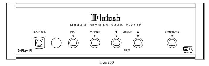
Front Panel Display Wi-Fi/NET LED Indicator changes color from Green to Red. Then release the two Push-buttons. The Power Save Mode is now Disabled.
