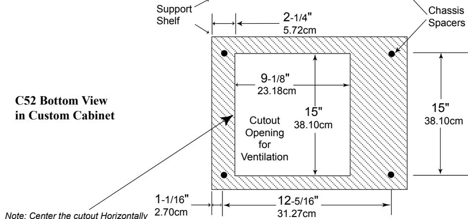
Note: Center the cutout horizontally on the unit. For purposes of clarity, the above illustration is not drawn to scale.
