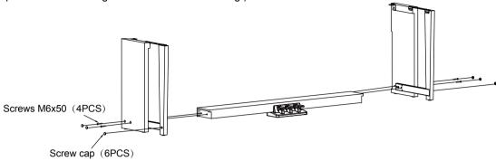
**B.** Place the Rear board ④ against the Legs, then insert the screws ⑥ through the holes and fit them into the Legs and foot pedal box.
