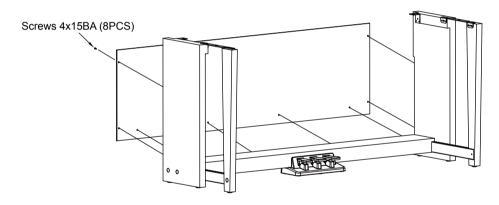
**C.** Place the Piano body on the stand, then fix it with the screws 9 & 0.
