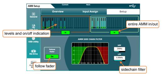
Like the '**Overview**' screen, this displays an overview of all AMM slots, with gain metering and indication of whether or not channels have AMM switched on.
