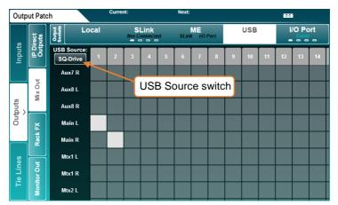
The 'USB Source' switch displayed at the top left of the patching matrix shows the current mode.
