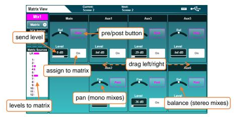
3) The matrix sends are shown on faders when a mix channel is selected and the momentary '**CH to All Mix**' key is pressed on the surface of the SQ.
