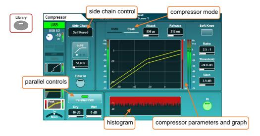
Switch the Compressor in or out using either the on-screen '**In**' button or the physical Compressor '**In**' key (to the left of the dedicated Compressor threshold rotary).
