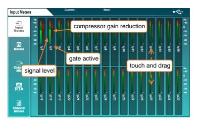
The first three tabs on the 'Meters' screen show 'Input Meters', 'FX Meters' and 'Output Meters'.
