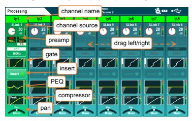
This gives the processing overview for 8 channels at once, with the selected channel highlighted. The view will automatically change if a channel is selected which is out of view, though you can also touch and drag to see all channels for the current layer. The selected mix channel is displayed to the far right.
