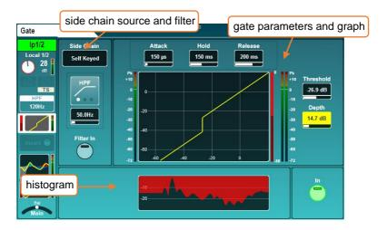
Switch the Gate in or out using either the on-screen 'In' button or the physical Gate 'In' key (to the left of the dedicated Gate threshold rotary).
