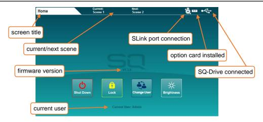
This is the first screen shown when powering on the SQ. It is also shown when no channels are selected, and '**Processing**' or '**Routing**' screen keys are active. The firmware version is displayed in the centre.
