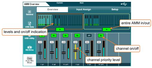
The top part of the screen displays an overview of all AMM slots, with the metering showing gain being applied to channels and indication of whether or not channels have AMM switched on.
