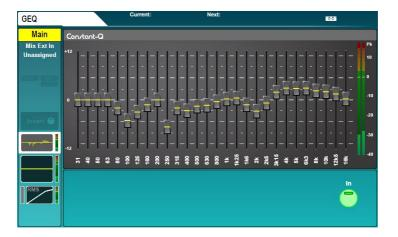
All mix channels feature a 28-band stereo graphic EQ. With a mix channel selected, and GEQ active, the green 'In' LED in the GEQ section (below the PEQ rotaries) will illuminate.
