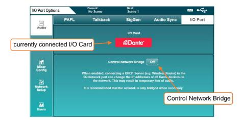
This screen shows which option card is currently connected. It also contains the 'Control Network Bridge' switch.
