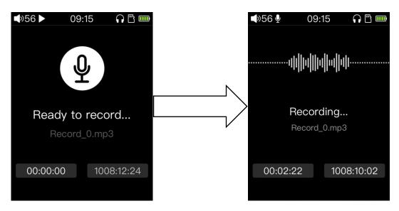
After clicking into the recording screen, the above picture will appear. At this moment, the recording does not start. Press the confirm button shortly to start recording. As shown in the right figure above, the status bar displays the recording icon.
