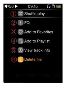
In the now playing screen, Shortly press the shortcuts button to enter the shortcuts menu screen, as shown above. Users can switch and operate some common functions through the shortcut menu Quickly.
