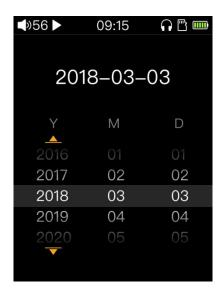
After entering this screen, the cursor will appear on the "Y" setting, as shown in Figure 1, move the cursor to the column to be adjusted, press the confirm button to enter the adjustment mode (the cursor turns yellow, as shown in Figure 2 above), and then touch by sliding Or press the previous/next button to adjust the corresponding date. After the setting is completed, press the back button to save the setting. (The same is true for the month and day settings)
