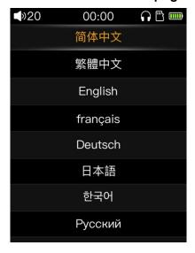
Press and hold the power button when M3 is off, it will start up in about 2s; when you turn on M3 for the first time, the language selection screen will appear. You can slide the cursor through the touch bar as needed, select the corresponding display language and press the confirm button to confirm and save you choice (You can also switch other languages in the system settings - Switch other languages). As shown in the figure above.
