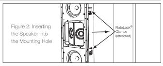
NOTE: THE ROTOLOCK® SYSTEM CAN ACCOMMODATE A WALL MATERIAL THICKNESS OF 1 1/4" (32MM). WITH THE TOGGLE FOOT CAP REMOVED, THE SYSTEM CAN ACCOMMODATE A WALL MATERIAL THICKNESS OF 1 1/8" (48MM).
