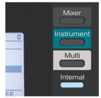
To assign a different preset to each of the buttons, press and hold [Internal] and select a preset using [E1/Data]. Now release [Internal]. The preset is loaded instantly upon release.
