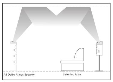
The A4 uses a concentric speaker design where a 1/2-inch tweeter resides in the center of a 4-inch midrange driver. The A4 speaker should be placed within ear level of the listener, preferably directly on top of your existing bookshelf or floorstanding speakers. The A4 should not be blocked by any object as the obstruction will greatly affect its performance and will degrade the effects it is trying to achieve.
