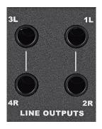
You can use these outputs for more than just speakers. If you want to use hardware outboard equipment, you can send out up to four mono, or two stereo signals from these outputs, This is configured in the iD mixer software.
