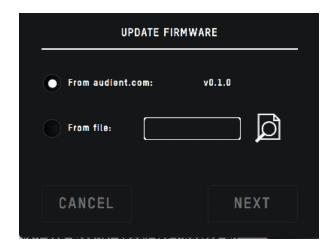
The latest version number will be retrieved from our servers and will be displayed (as shown above). Press next to continue with the firmware update. Press 'update' to install it. Once complete reboot iD44 using the power switch to apply it.
