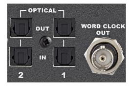
Running in S/PDIF mode, the optical i/o provides the option to integrate external digital outboard, allowing upto 4 channels of audio in and out of the iD44 at sample rates up to 96KHz.
