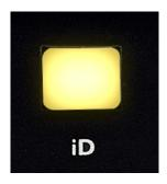
The iD button switches iD44 into ScrollControl mode, allowing the encoder to be used as a scrollwheel for the computer. This gives you the ability to control plugin parameters and anything else that is scrollable. This works well for adding automation or setting parameters in a hands-on way.
