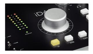
Accompanied by this monitor volume knob are permanently assigned hardware DIM & CUT switches. The level of DIM and ALT. loudspeaker trim can be adjusted in the iD mixer application.
