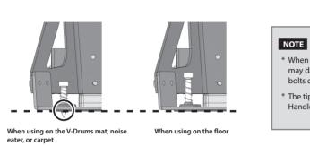
\* When used on flooring, the anchor bolts may damage the floor. Adjust the anchor bolts correctly.
