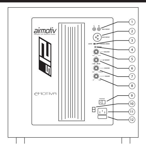
All of the controls and input connections on the Airmtoiv S10, S12, and S15 are on the rear panel. All three models offer the same input and control options (the Airmotiv S12 is shown).
