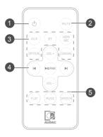
1) Power button: Switches the sound bar between ON and STANDBY mode.
