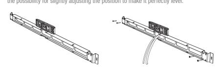
Make sure the appropriate fasteners are used, depending on the mounting surface (brick, concrete, wood,  $\dots$  )
