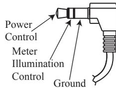
*Note: When it is desired to switch Off the green illumination of the Small Signal Tubes, and the MC275 is not connected to a McIntosh McIntosh Preamplifier or A/V Control Center with meter illumination control, connect a 1/8 inch Mono mini phone plug to the POWER CONTROL IN jack.*
