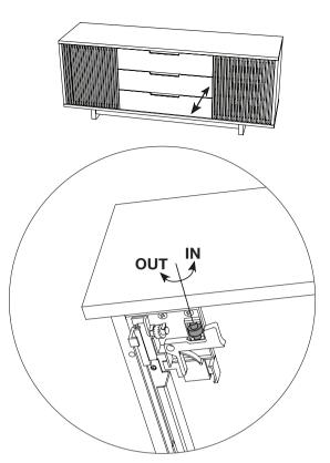
Front-to-Back Adjustment: Turn Black Wheel on one or both mechanisms, as necessary, to adjust drawer position in or out.
