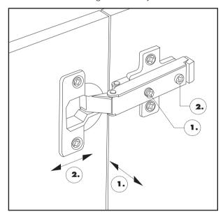
Use the supplied **Phillips Screwdriver (A)** to adjust Vertica's door hinges:
