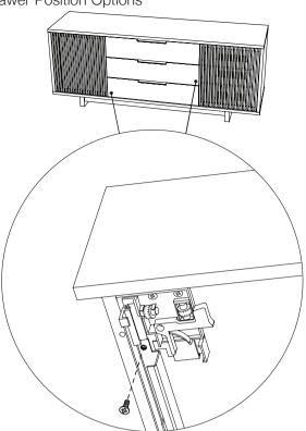
Two (2) adjustment mechanisms are found on underside of each Vertica drawer, at left and at right. All drawer position adjustments require removal of indicated screw on both adjustment mechanisms. Save screws for re-installation prior to any future cabinet shipment.
