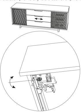
Lateral Adjustment: Turn White Wheel on both mechanisms to adjust drawer position left or right.
