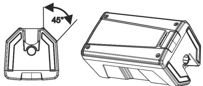
The rear side inclination, symmetrical, as shown in the upper picture, is 45°. The related wedge positioning is shown in the picture. B-HYPE can be used as a stage monitor in small contexts, in this case please consider the characteristic dispersion pattern presented above.
