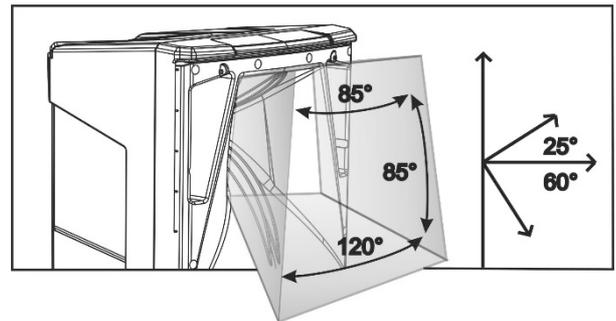
The acoustical design allows to face different environments. The dispersion pattern is asymmetrical on the vertical axis, and the horizontal coverage varies within position: It is wider in the lower side and narrow in the upper one.
