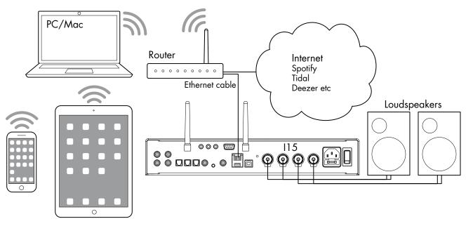
The 115 can use Chromecast to connect directly to a music service that supports Chromecast, such as Spotify, Deezer, Tidal, or Tuneln Radio. The music is streamed direct to the 115; once set up you can use your phone to make calls, or play other audio.
