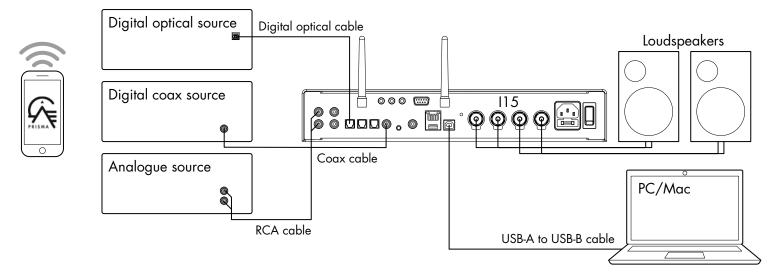
These methods of playing music from the 115 involve connecting the source to the 115 via a cable, and don't require Wi-Fi, Ethernet, or Bluetooth.
