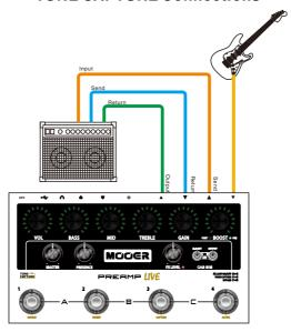
The amplifier must have an effects loop or "preamp out" to work. It must have a speaker load connected at all times during the capture process. DO NOT connect the speaker output of your amplifier to PREAMP LIVE.
