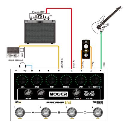
When the effects loop is set to MODE A (SERIAL) the POST NG will be before the effects loop.
