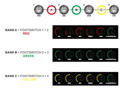
The colour of the CHANNEL CONTROL LED's will indicate which BANK is currently selected. After selecting a different bank the PREAMP LIVE will wait for you to select a channel within that bank before changing the sound.
