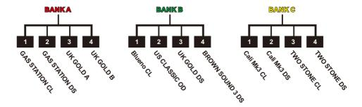
The channel selection logic of PREAMP LIVE is based on the same control methods you might find on a traditional 4 channel tube amplifier.
