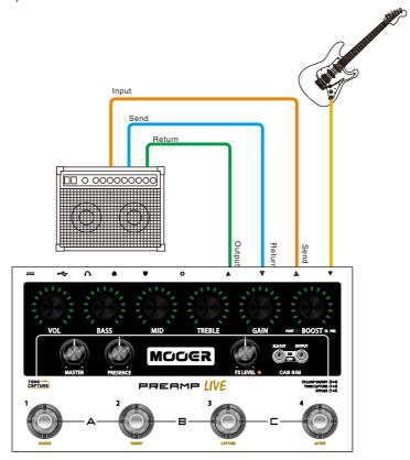
When the effects loop is set to MODE B (A/B) the POST NG will be after the effects loop.
