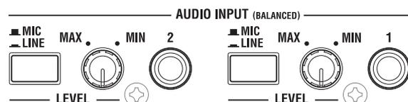
Inputs 1 and 2 provide 1/4” TRS balanced connectors. You can use these for either microphone-level or line-level signals. The two inputs have identical sets of controls, as described below.
