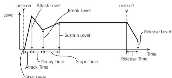
The HD-1 includes three EGs, for Pitch, Filter, and Amp. These produce time-varying changes in pitch, tone, and volume respectively. They can also be used to modulate a number of other Program parameters via AMS.
