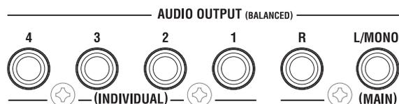
Connect these outputs to the input jacks of your amp or mixer. In addition to the L/MONO and R main stereo audio outputs, the KRONOS provides four individual audio outputs.
