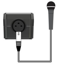
Move the Power switch to the ON position. If you have connected a condenser microphone, select the +48V position to supply phantom power. The 48V LED on the front panel will light red.
