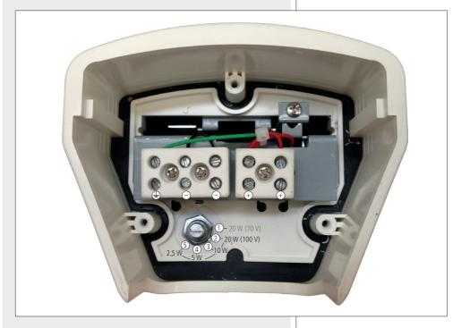
Connections with the audio line are made by using the internal ceramic screw terminal strip (it is necessary to remove the bottom cover by loosening its three screws). The + / - terminals allow to connect both input and output cables (to link other loudspeakers in parallel).
