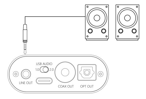
Iine out is controlled by the power/volume knob and can work with 2.5mm/3.5mm output at the same time; but recommend to eject the 2.5mm/3.5mm headphones while using the line out.
