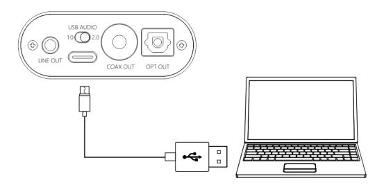
USB Audio 1.0, decoding sampling rate can reach 96k/24bit, no need to drive
