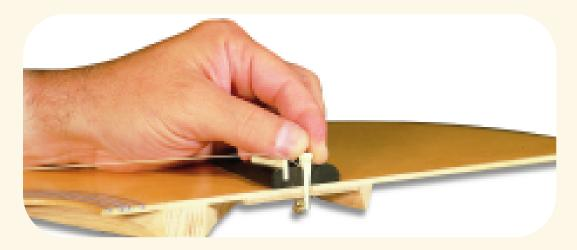
You might occasionally encounter an older guitar with a thin bridge or a string with a longer double winding adjacent to the ball end. Shown above is an old luthier's trick or remedy. An extra ball from an old string is placed over the string and drawn against the first ball. This will effectively back the string into the bridge, removing the heavy area of the string from direct saddle contact.
