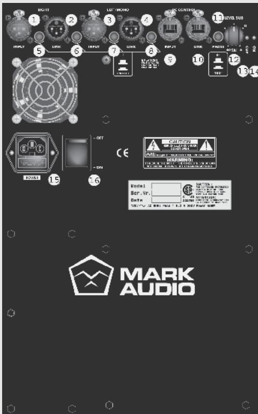
**INPUT RIGHT & LEFT/MONO (1-3)** - Line input jacks for connecting stereo audio sources. The XLR 3-pole female jacks are electronically balanced (hot pole #2). You can use unbalanced sources if your cables have pole 3 jumpered with pole 1.
