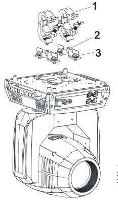
1.Clamp 2.Omega-holders 3.Quick-lock fastener
