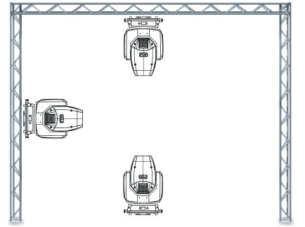
The Vizi Hybrid 16RX is fully operational in three different mounting positions, hanging upside-down from a ceiling, sideways on trussing, or set on a flat level surface. Be sure this fixture is kept at least 12m (40ft) away from any flammable materials (decoration etc.). Always use and install the supplied safety cable as a safety measure to prevent accidental damage and/or injury in the event the clamp fails (see next page). Never use the carrying handles for secondary attachment.
