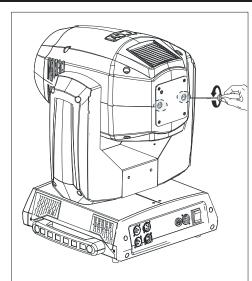
Replacing the lamp is relatively easy. Unplug the unit from its power source. Allow the unit 15 minutes to cool down. Start by unscrewing the two phillips screws that hold the lamp door in place. **DO NOT UNSCREW THE SCREW LOCTATED ABOVE THE MAIN SCREWS!**
