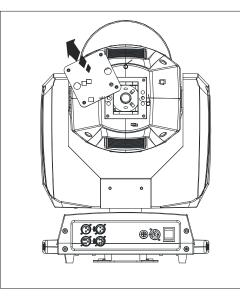
Pull the lamp door out and rotate to the side as the diagram shows. You will not have access to the lamp.
