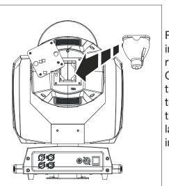
Replace the lamp by placing the new lamp into the right side lamp "sleeves". Once properly placed in the "sleeves", gently slide the lamp to the right. Once the lamp is to the right, the lamp can now be placed into left side "sleeves"
