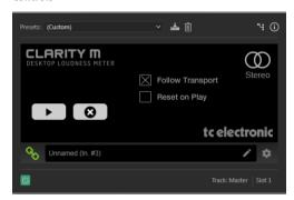
Click the Play/Pause icon to manually start and stop the metering. This button overrules the 'Follow Transport' function. Click RESET to perform a manual reset of the meter.
