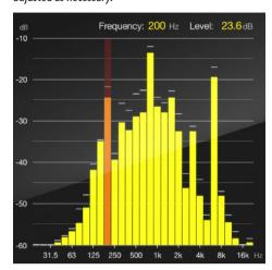
Press the 1st button to automatically set the scale top values of the level scale (dB) of the RTA view according to the current audio source. Alternatively, both scale range and scale top values can be set automatically (see Chapter 7, callout 12). Setting the scale automatically will give you the best visual feedback and ensure that certain frequencies aren't rising beyond view. Note that this is only effective while audio is being played.
