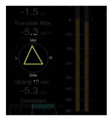
The top of the triangle will point toward the top/center of the semi circle when a perfect left-right balance is achieved. The width is indicated by how broad the base of the triangle is.
