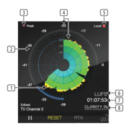
Press the 1st button to start or pause the loudness measurement. True-peak and correlation will continue to be measured. The 2nd button provides a global reset, and will reset all values across Clarity M. By default, the rotary knob adjusts the radar speed, but can be changed to adjust resolution or target loudness in the System (SYS) menu.
