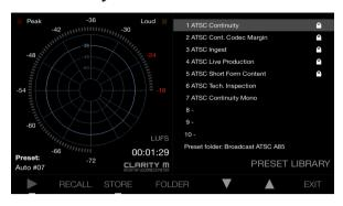
Presets are composed of parameters found on the Edit page. Both RTA and Radar parameters are stored in a preset. Press the 4th button to access the Library menu. Scroll through the available folders with the rotary knob to select the most appropriate category.
