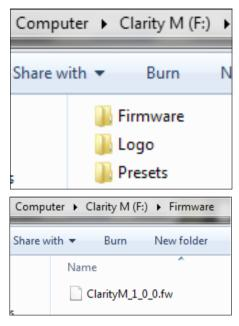
Navigate to the firmware folder and drag the new firmware file into the folder. The Clarity M should automatically detect the new file.
