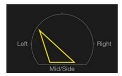
The top point will tilt either direction as the channels become less balanced, and the base will appear narrower to indicate less width.
