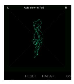
Identical stereo channels (mono) will appear as a straight line, and any stereo separation will visible as a deviation from this line.
