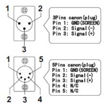
connector pin designations shall be as follows pin1:signal common(shield)
