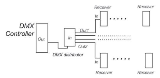
You can run a maximum of 32 units (receiver) per output channel.
