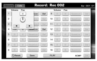
Press the "Quantize" button to call up a pop-up box showing the quantize accuracy. Use the DATA DIAL, the [+] or the [-] button to adjust the parameter.
