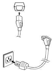
2 Connect the power cable to the AC power jack on the rear panel.
