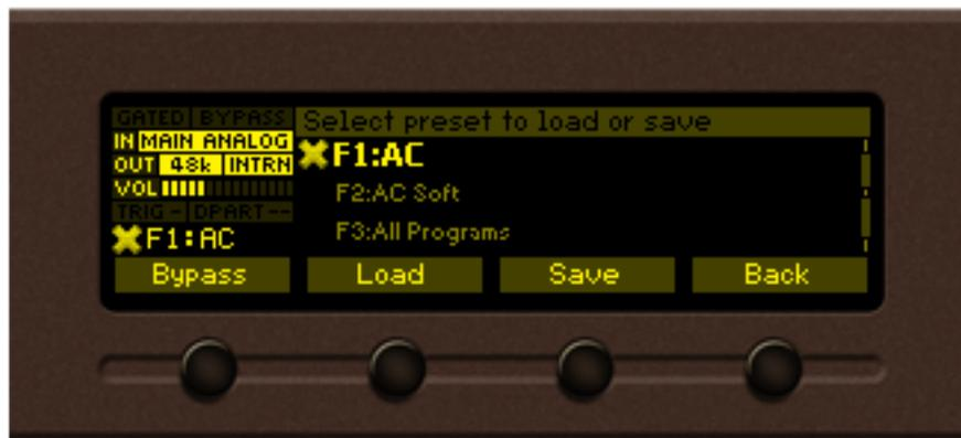
4. In order to save the changes, using the front panel keyboard, select one of the user presets then press the [Save] button. A window requiring verification will appear. Confirm the changes by pressing the [OK] button. The newly created preset will be automatically chosen as 'active preset'.
