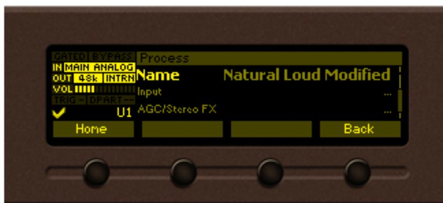
Specifying the new preset name is mandatory. If not, the DB64-FM will not assign a name and the newly created preset will be saved as U10 : DANCE (for example, if a factory preset is used as a basis) or U7 : -empty- (if user preset is used as a basis).
