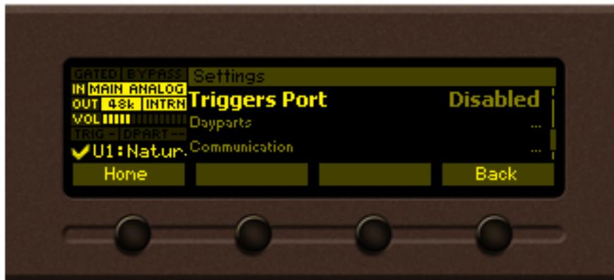
If enabled the remote trigger port will allow you to select any of the first 8 user presets by pulling one of the 8 pins on the trigger port socket. If more than one pin is triggered at the same time, the pin with the lowest number will be with highest priority. For example, if all pins are pulled low, trigger 1 will be with highest priority.
