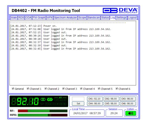
This screen shows the Device Log, which shows the last 100 important events. Selecting/deselecting the corresponding check-boxes will filter the events by type.
