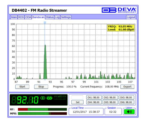
This Screen evaluates FM broadcast band congestion by sweeping the tuner across the FM band, logging every carrier and generating a spectrum display of carrier level vs. frequency.
