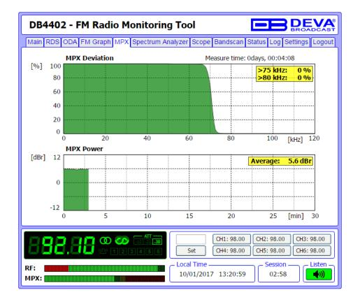
The MPX page shows the baseband MPX deviation as a function of deviation in kHz over the observation period. The graph immediately shows modulation density.
