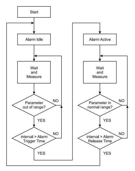
**Block Diagram of Alarm Automata**
