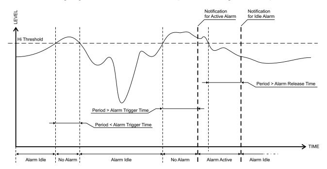
If RDS Group has not been received for more than Alarm/Warning Trigger Time state is changed to Active. If state is Active and Release Time has elapsed and the RDS Group is received state is changed to Idle. If the RDS Group is received before the Release Time is elapsed state remains Active.
