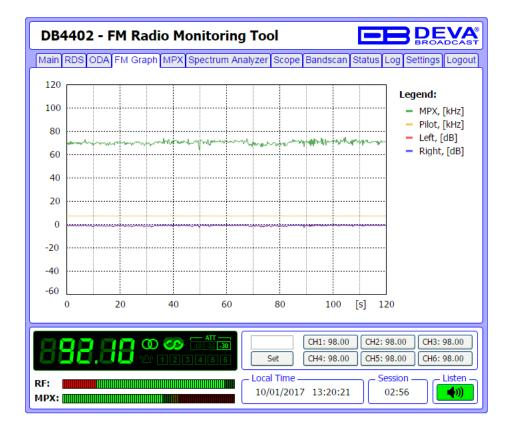
The FM graph is a multi-colored plot of MPX, Pilot, Left and Right audio levels. These mandatory parameters are represented in the time slice of 2 minutes, ensuring reading at a glimpse all significant parameters of the analog signal. Each parameter has its own color representation and measurement units, which are indicated on the right-side of the graph. When RDS mode is selected, the MPX and PILOT readings are in kHz. When RBDS mode is selected, the readings are in %.
