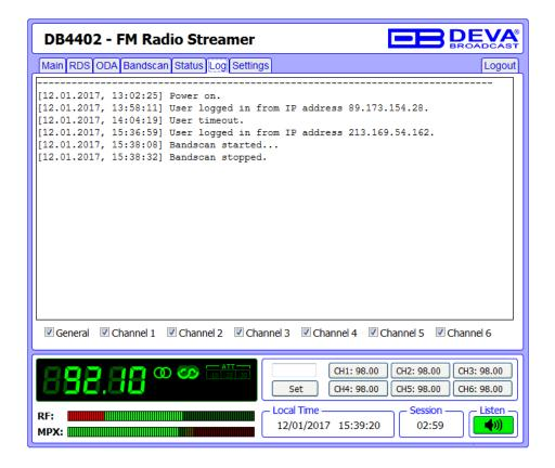
This screen contains the device's Log, which shows the last 100 important events. Selecting/deselecting the corresponding check-boxes will filter the events by type.
