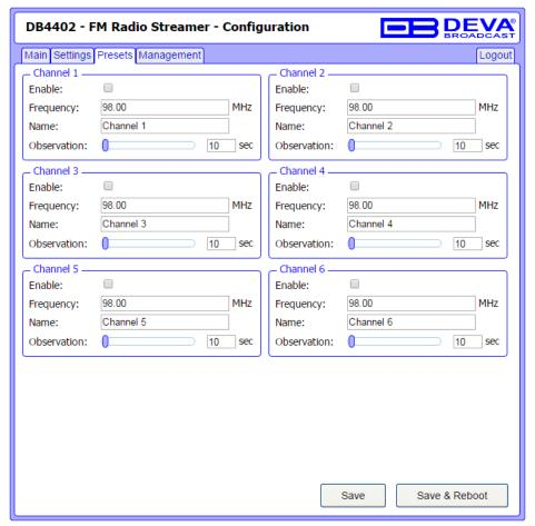
Presets tab allows the frequency presets and audio stream to be configured. The FM streamer works on a rotation principle. Each of the enabled and set channels will be included in an uninterrupted audio stream that could be heard using suitable audio player (Media Player, Winamp, etc.) or through the WEB interface by pressing the [Listen] button. The Audio Stream Server is configured in **Settings > Audio**, "Main Settings Screen" on page 49.
