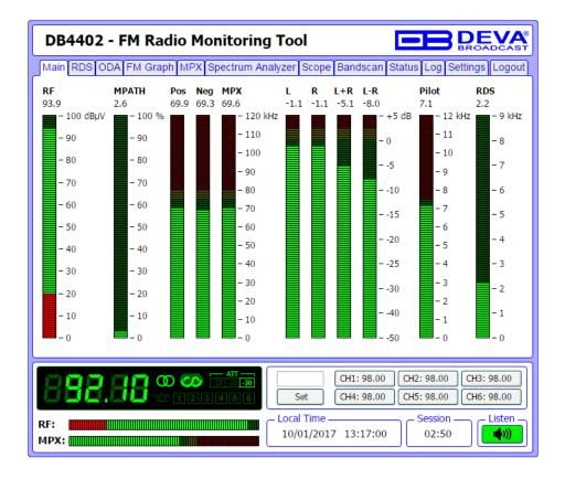
The main page shows meters for RF level, measured multipath level, baseband modulation (positive and negative peaks), audio levels, PILOT and RDS/RBDS levels.
