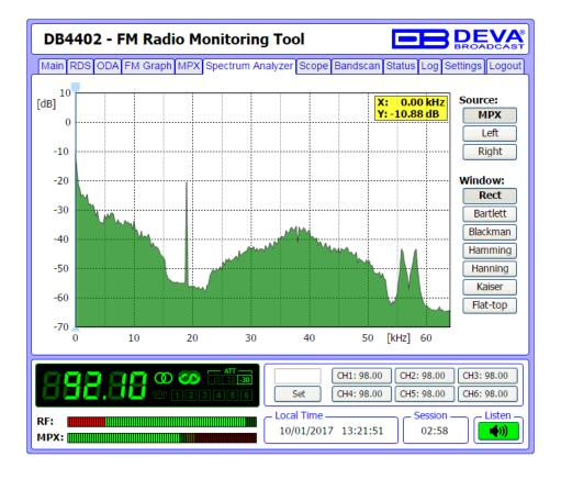
The spectrum analyzer tab is a very useful feature: It is a MPX and audio spectrum display. Initially it shows the MPX from 0-65kHz so that the readings of the currently selected source (composite MPX or stereo Left/Right) to be clearly visible. The signal source to be calculated and visualized is chosen from the Source section placed on the right part of the screen. Spectral components of the selected signal are determined on the base of Fast Fourier Transform.
