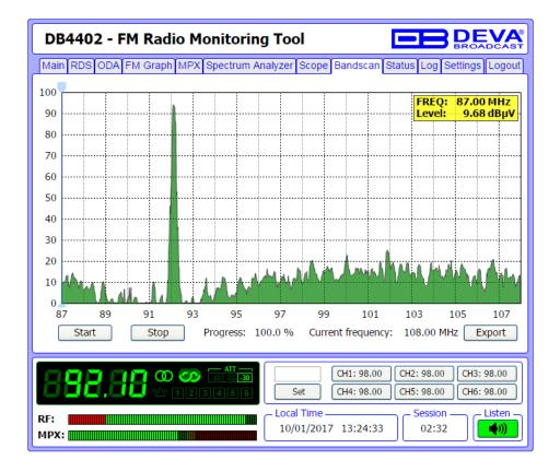
This Screen evaluates FM broadcast band congestion by sweeping the tuner across the FM band, logging every carrier and generating a spectrum display of carrier level vs. frequency.
