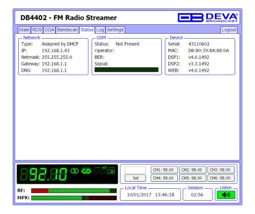
Information on the basic device and network status (IP address, MAC, etc.) is available in this section. If a GSM modem is connect to the DB4402, information on its current status will also be available.
