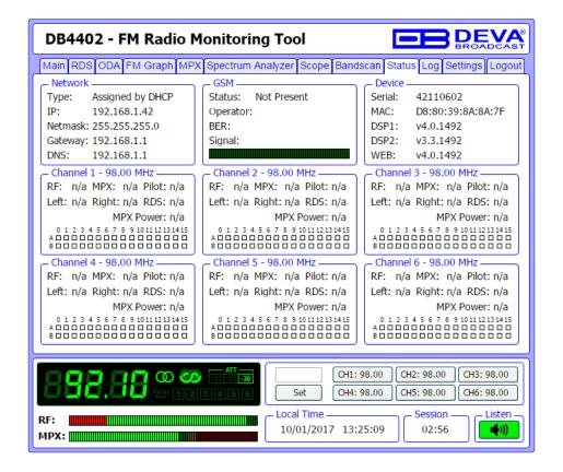
The status tab shows the alarm status of each parameter of the preset frequencies, along with the basic device and network status (IP address, MAC, etc.).
