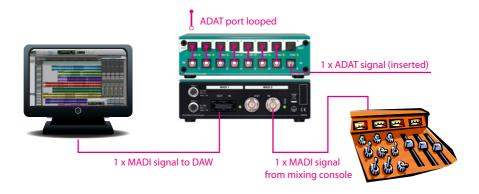
A slight delay of three samples is introduced on **each** I/O. So, in this example the latency between MADI input and MADI output adds up to six samples in total. All devices must be in sync to each other.
