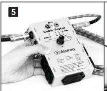
Test cable (two): twist the knob to the position of "2" and "3", if the LED light on one by one, it indicates that PIN-2 and PIN-3 of this line is well. If the light is crossover light on or one light is not light on, it indicates there is something wrong with line.
