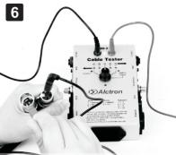
The application of probe line: insert two probe lines into banana jacks, if you hear buzzing and yellow LED light on, it indicates that the line is well. According to this method, to test audio cable which the inserting holes are not matching. Use probe pen to connect audio cable, if you hear buzzing it indicates that the line is well.
