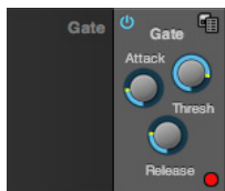
Figure 8-2: The Gate module.
