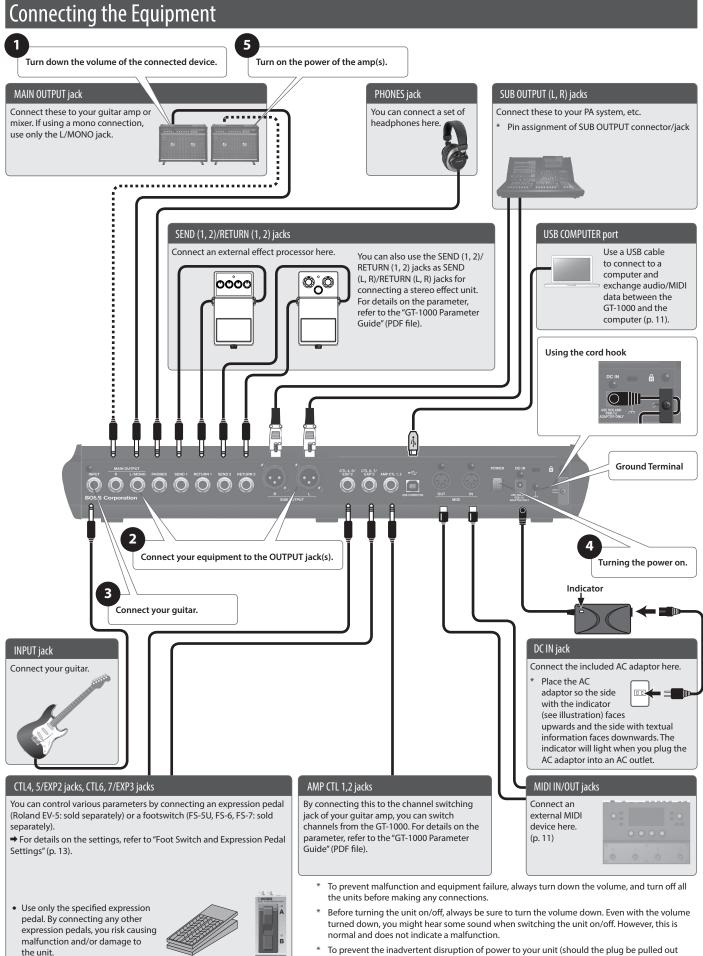
\* To prevent the inadvertent disruption of power to your unit (should the plug be pulled out accidentally), and to avoid applying undue stress to the jack, anchor the power cord using the cord hook, as shown in the illustration. In this manual, the order of the MENU operations is written as follows.
