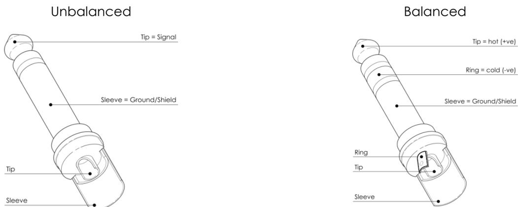
For these applications the unit provides 1/4" TRS and XLR connectors to easily interface with most professional audio devices. Follow the configuration examples below for your particular connection.
